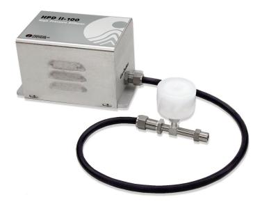
The HPD II reduces the pressure of dry, inert, non-toxic, non-flammable gases, such as Clean Dry Air (CDA), nitrogen, carbon dioxide and argon to a level acceptable for the Lasair II 110 and Lasair III 110 aerosol particle counters, which are designed to operate at atmospheric pressure.
